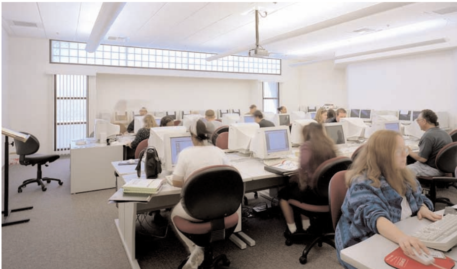
Computer Science Laboratory at Antelope Valley College, is a good example of controlled lighting using glass block and vertical windows and sun walls adjacent to the windows to provide diffused light.
