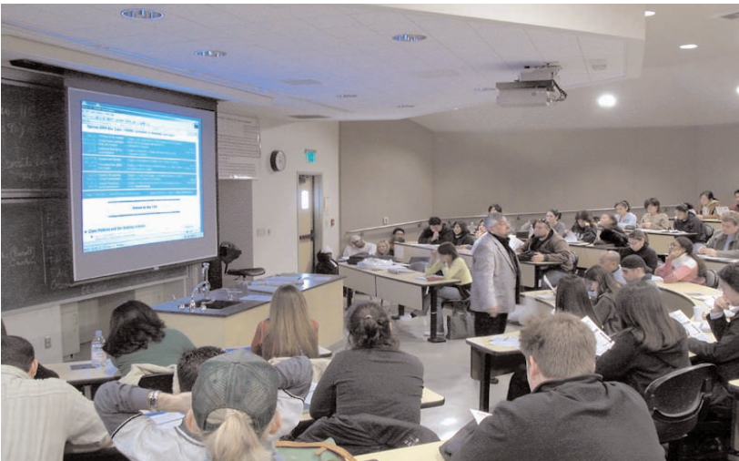
Glendale Community College science lecture hall with integrated network connections for web-cast lectures, adequate equipment for digital instruction, stepped sitting with internet access for laptop computers, sloped ceiling for better acoustics and controllable lights.
