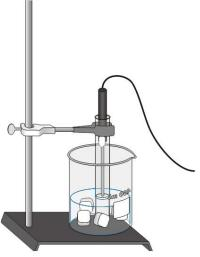
3. Prepare your cooling mixture by placing about 150 mL of ice in a 250 mL beaker; then add water to barely cover the ice.
